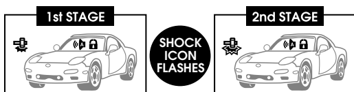
FIG-6: Pager LCD Icon Change Upon Shock Detection
